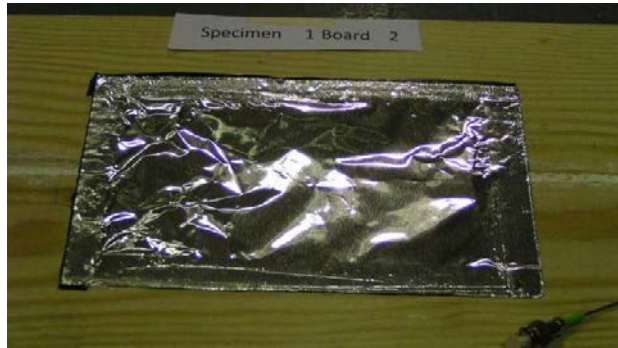
(b) Aluminum foil package bonded with tape
