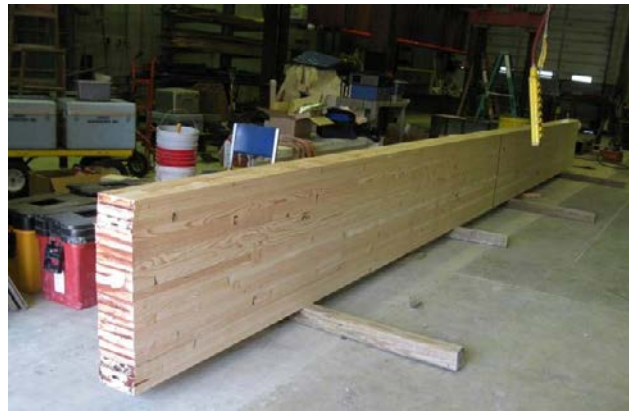
Figure 6.97: Full Scale Glulam Girder at the Laboratory
