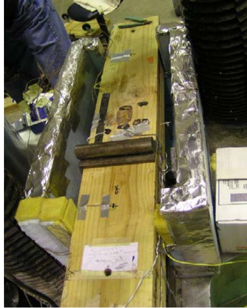
Figure 6.30. Cold and Sustained Loading Test: Placing the Specimen in the Cold Box
