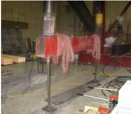
(a) Steel frame with hydraulic jacks
