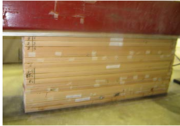
(b) Pressing of the glued laminates
