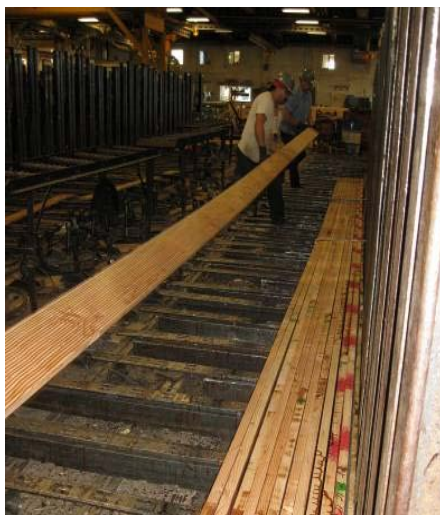
(c) Manually placing one laminate L3
