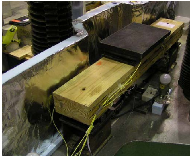
Figure 6.27. Heat and Sustained Loading Test: Assembling of the Heat Box
