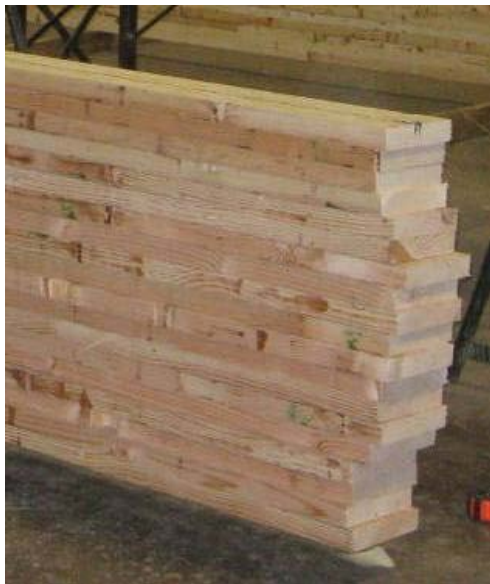
(a) Selected laminates for girder assembling
