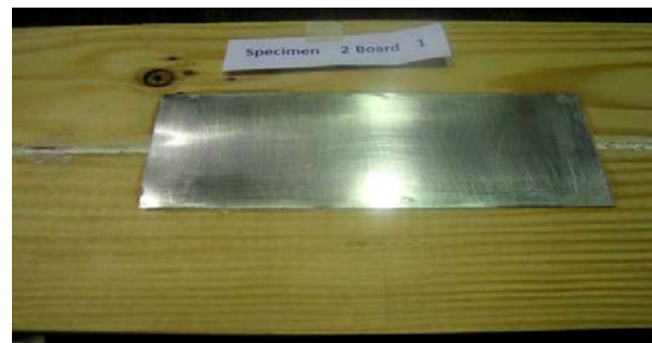
(b) Steel shim bonded with adhesive
